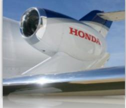
Unlike most jets, Honda's design mounts the engine above the wing-which will allow for drag reduction, noise reduction, and fuel efficiency, according to the company.
